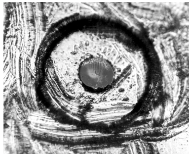
Figure 5-6. Damage from improper cleaning.
